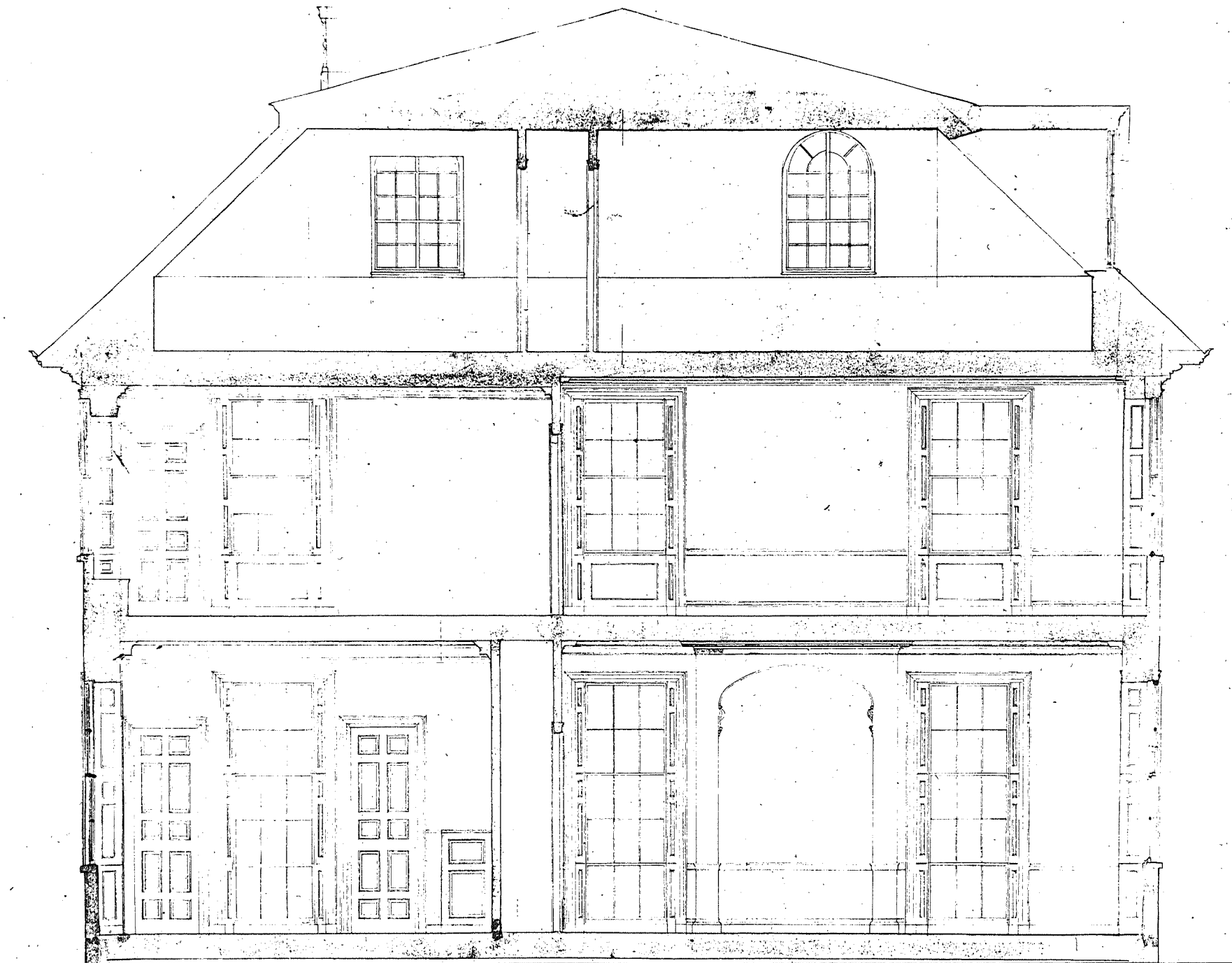
Fig. B-13. Section Looking North, ca. 1890, by Ogden Codman, Jr. Architect, showing Dining Room sideboard alcove and decorative plaster work. (Codman Collection of Architectural Drawings, SPNEA)
